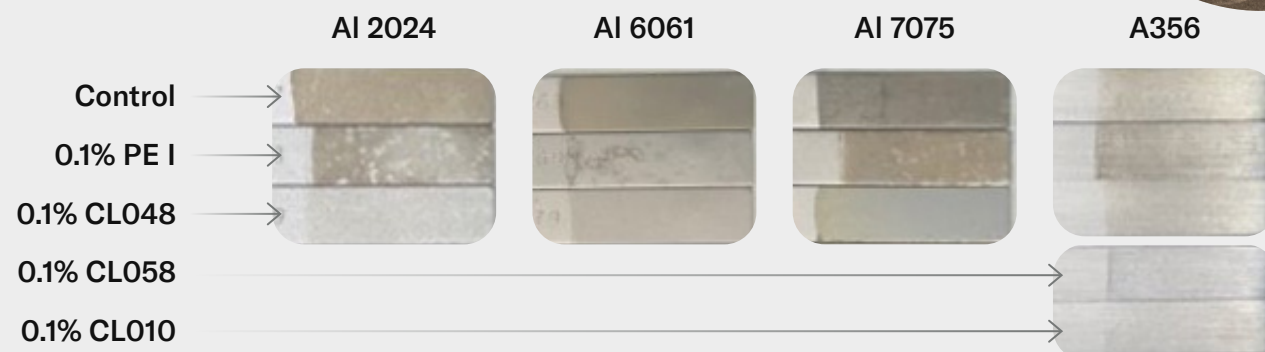
Figure 3. Various coupons after treatment with Solugen products vs. PE I
