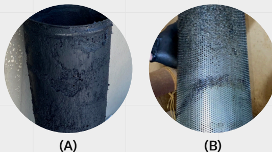
Figure 1. SWD Inlet Filter (A) before Verza application and (B) after Verza application.
